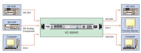
Figure 1. Using the VC-300HD various video formats can be acquired as HDV or DV.
